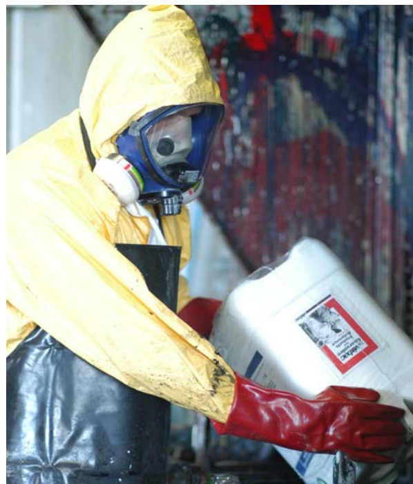
Figure 1 – the powders, resins, solvents and additives used in coatings and ink manufacture must be handled in controlled conditions in order to protect workers and the environment
